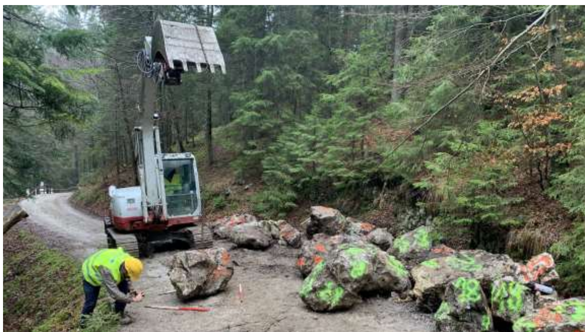
Figure 75: All the rocks have been numbered in order to be recognised during each simulation.
