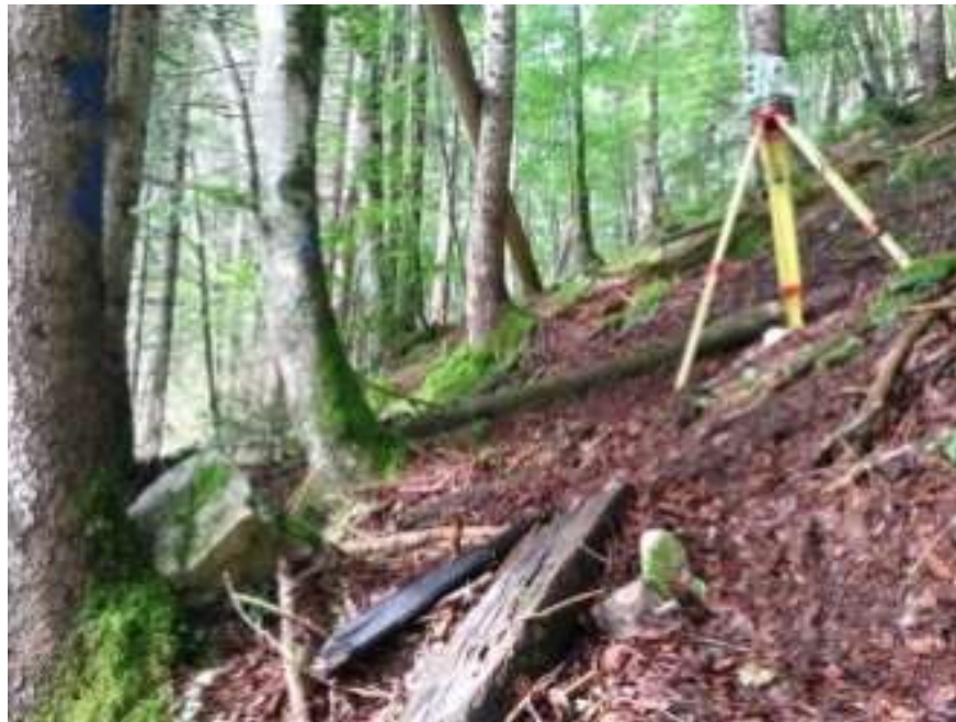
Figure 40: Leica MS50 MultiStation scanning the forest.
