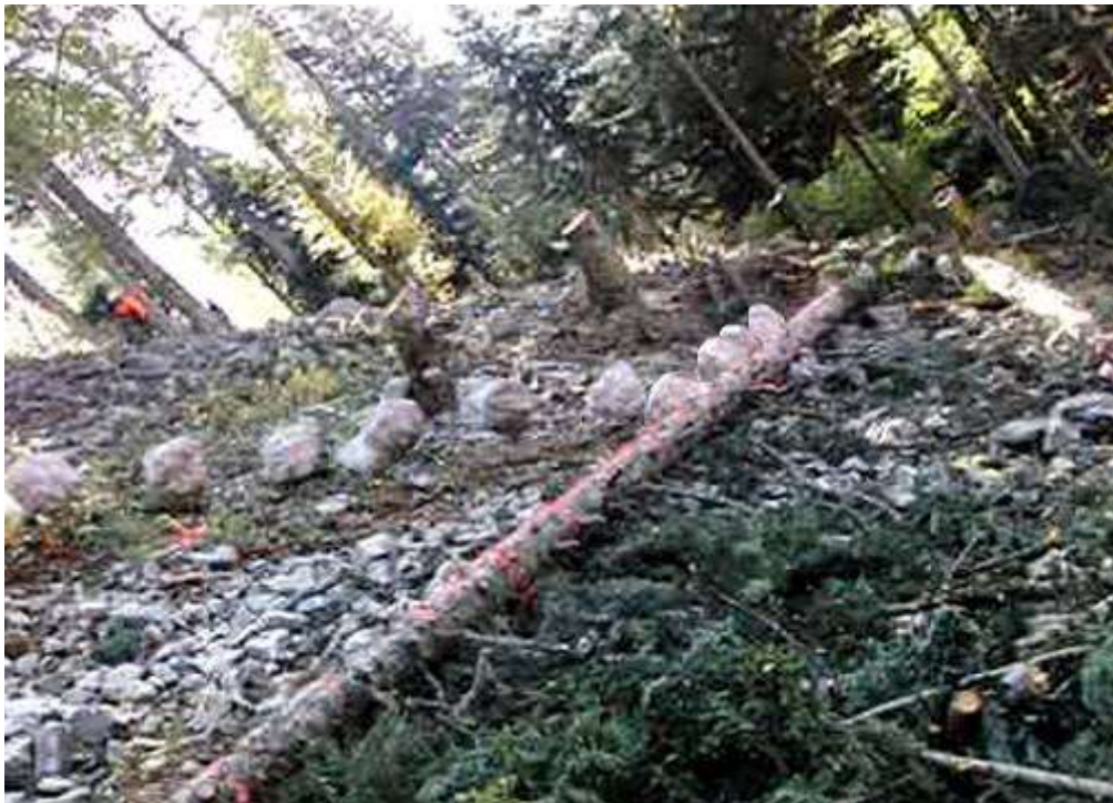
Figure 14: Single-frame sequence of a log blocking a rolling stone (photo: IRSTEA).
