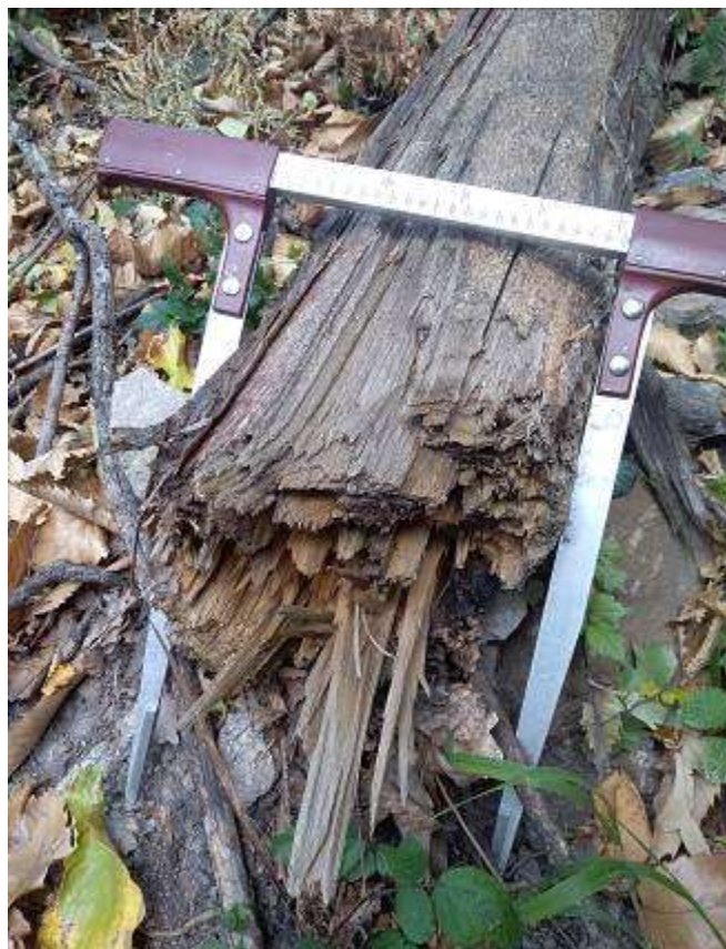
Figure 13: Chestnut stem neatly broken by the passage of a big rock (Cervo, Italy).
